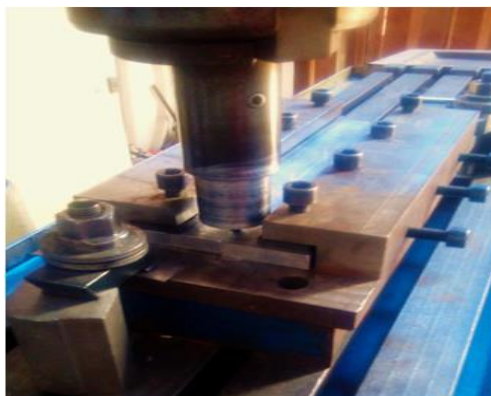
Fig. 1 Friction stir welding process.
