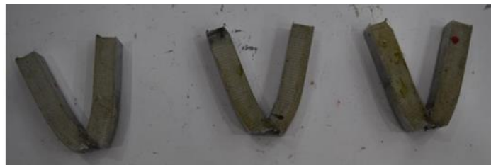
Fig. 4. Sample of maximum Impact Energy = 89.99 Joule at Room Temperature with Tool Rotational Speed = 740 RPM, and Welding Transverse Speed = 31.5 mm/min.
