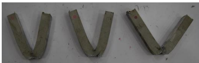
Fig. 5. Sample of maximum Impact Energy = 98.66 Joule at Room Temperature with Tool Rotational Speed = 590 RPM, and Welding Transverse Speed = 31.5 mm/min.
