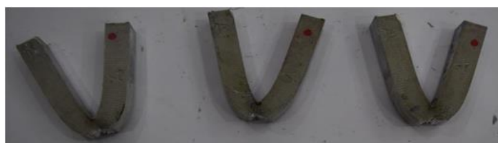
Fig. 6. Sample of maximum Impact Energy = 98.66 Joule at Room Temperature with Tool Rotational Speed = 470 RPM, and Welding Transverse Speed = 16 mm/min.
